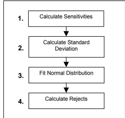
Figure 2: Steps of the Linearized Method
