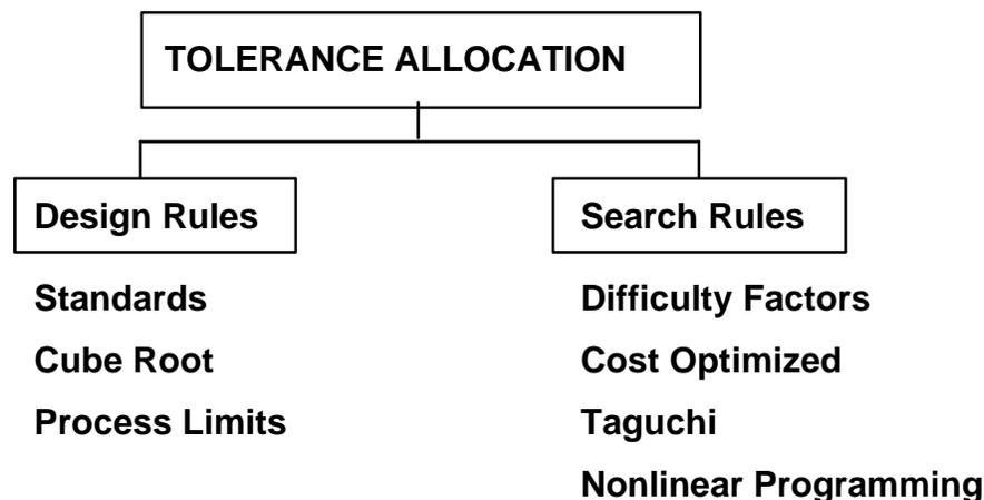
Fig. 7. Tolerance allocation methods.
