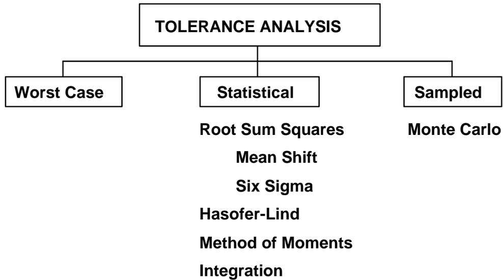
Fig. 2. Mathematical models of tolerance accumulation.
