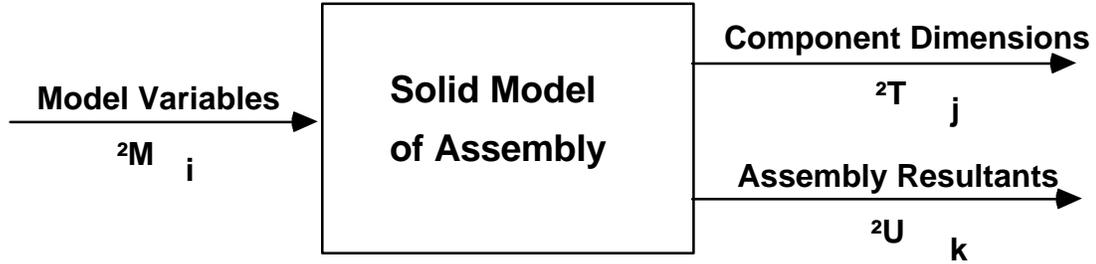
Fig. 4. Computing tolerance sensitivities from the solid model of an assembly.
