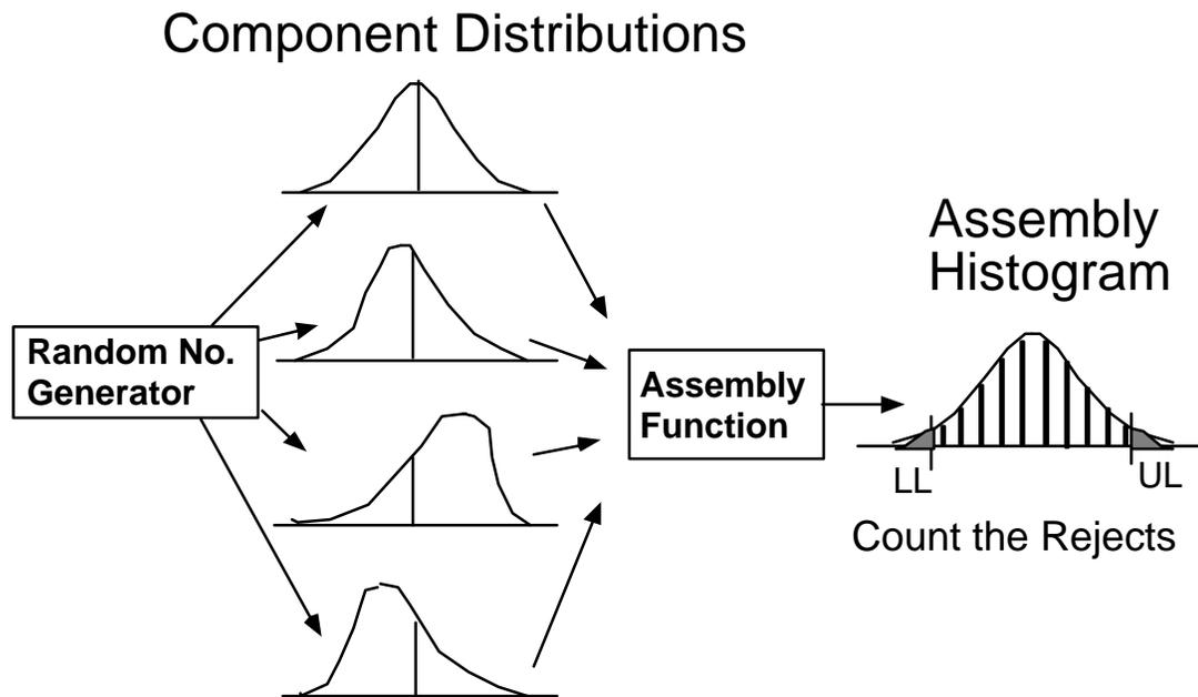
Fig. 5. Assembly tolerance analysis by Monte Carlo simulation.
