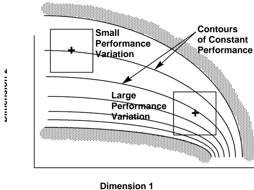
Fig. 8. Sensitivity reduction by shifting the nominal values.
