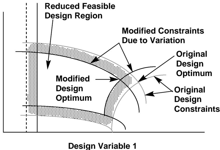
Fig. 9. Change in optimum and decrease in feasible region to insure design will remain feasible to variation caused by tolerances.
