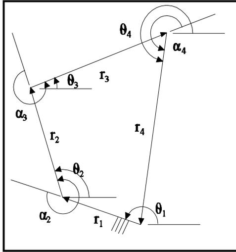
**Figure 2.3** A vector loop with relative angles used in the tolerance analysis of a four bar.
