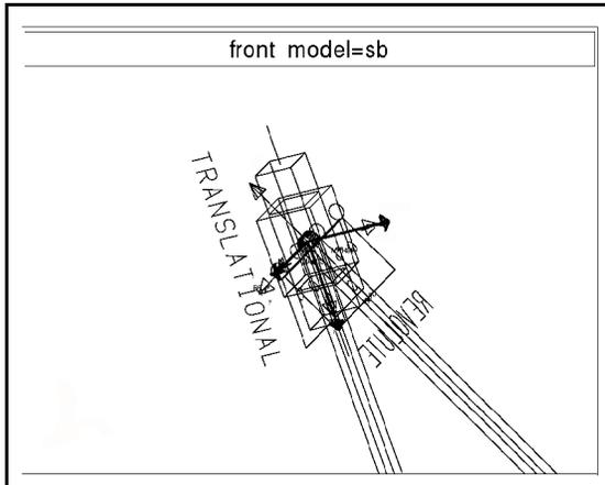
**Figure 5.11** A representation of a revolute joint in ADAMS.
