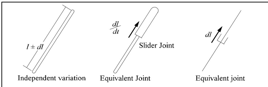
**Figure 4.9** Equivalent joints used to represent independent length variations
