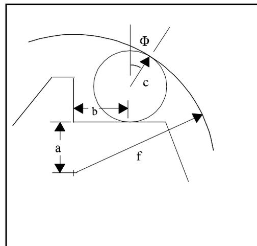
**Figure 3.2** Relevant dimensions for the clutch.
