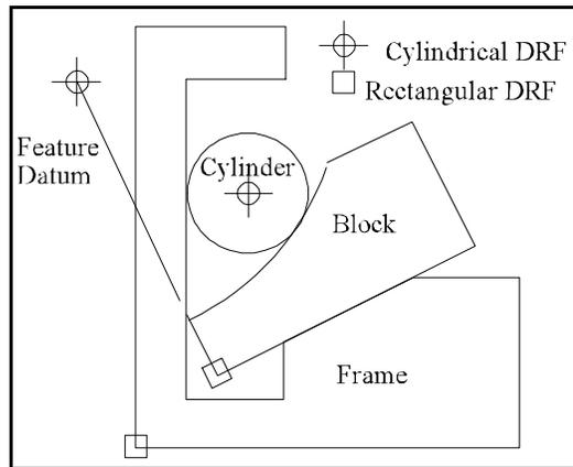
**Figure 4.4** Part and Feature Datum Reference Frames.
