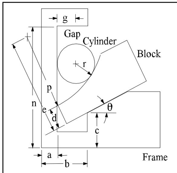
**Figure 4.2** The stacked blocks assembly and its dimensions.
