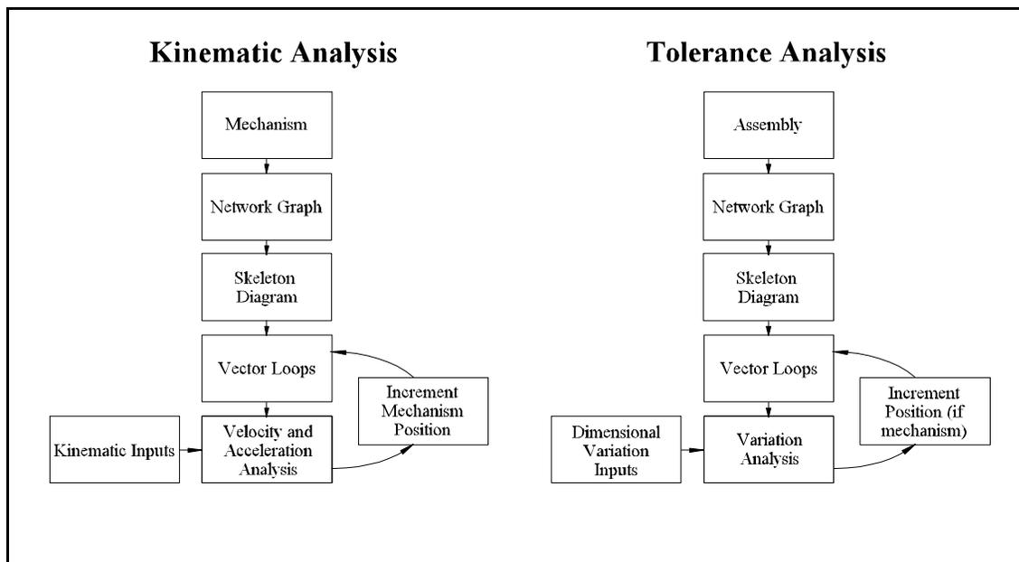
**Figure 4.1** Procedures for kinematic and tolerance analysis.
