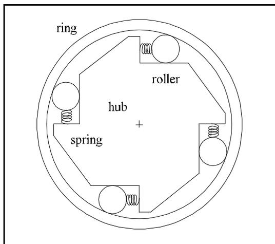
**Figure 3.1** One way clutch assembly.
