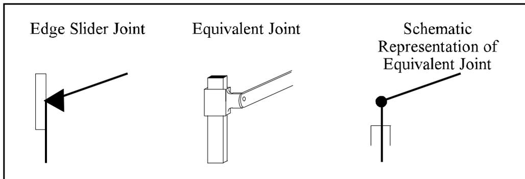
**Figure 4.14** The equivalent joint for the edge slider
