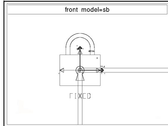
**Figure 5.12** Representation of a fixed joint in ADAMS.
