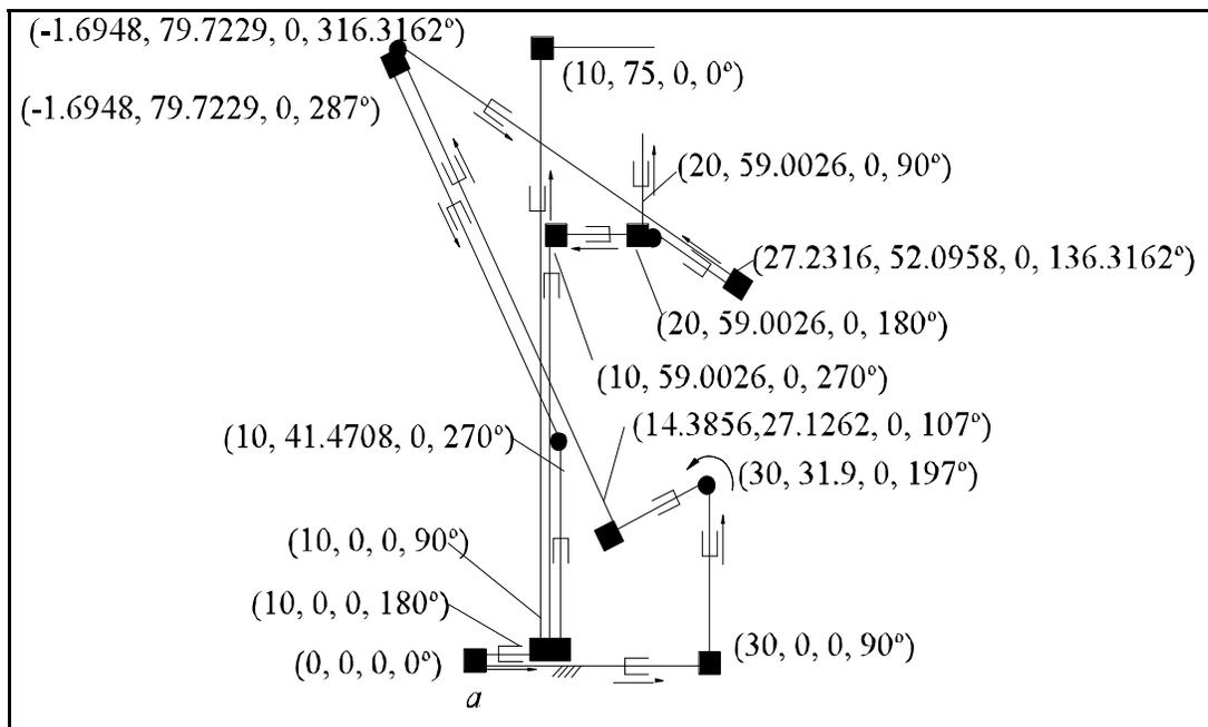
**Figure 5.3** Position and orientation of the links (x, y, z,  $\theta$ ).
