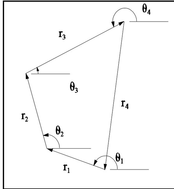
**Figure 2.5** The vector loop used in the kinematic analysis of the four bar.
