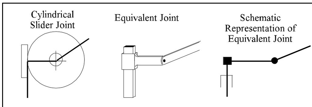
**Figure 4.13** The equivalent joint for the cylinder slider
