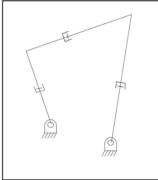
**Figure 5.14** Equivalent variational mechanism for the four-bar linkage.
