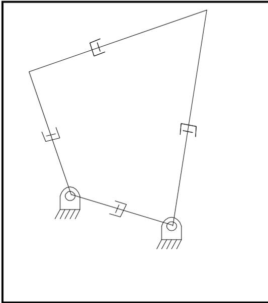
**Figure 2.4** A four bar mechanism with 'growing links'.
