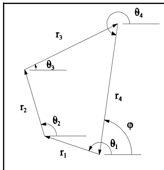
**Figure 2.2** The vector loop used in the kinematic analysis of the four bar.
