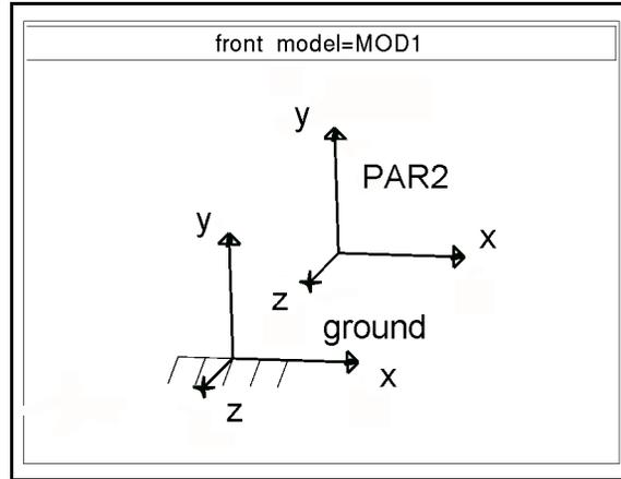
**Figure 5.7** A part in ADAMS, located with respect to the model.
