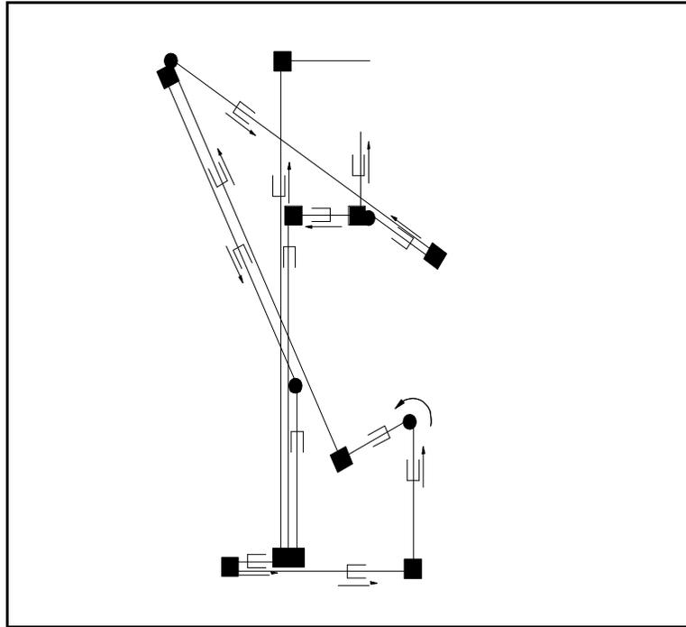
**Figure 4.17** Placement of fixed joints on the stacked blocks assembly.
