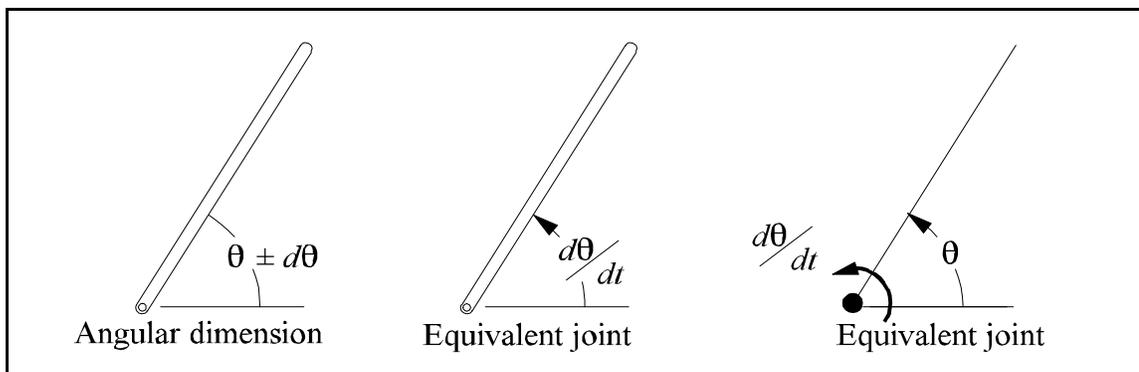
**Figure 4.10** Equivalent joints used to represent independent angular variations
