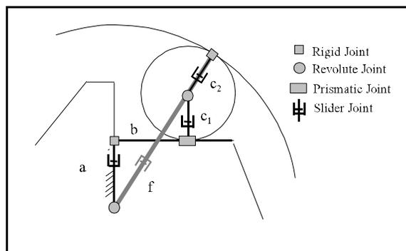
**Figure 3.4** A mechanism variationally equivalent to the one way clutch.
