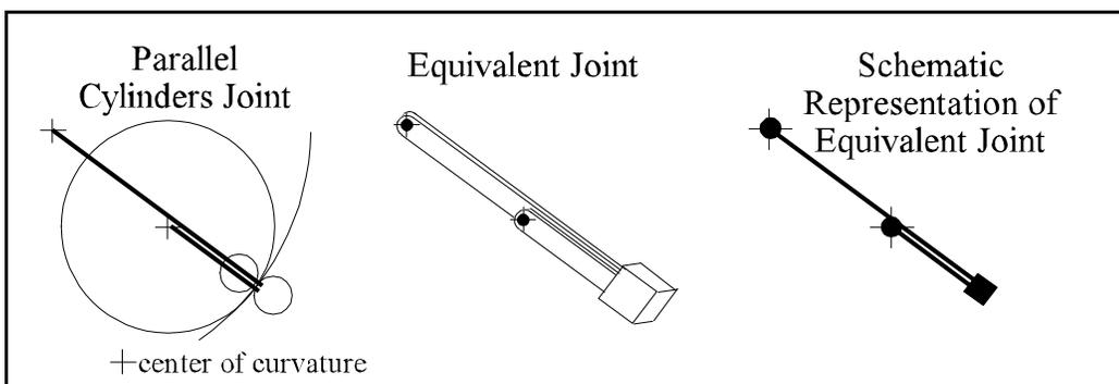
**Figure 4.15** Equivalent joints for the parallel cylinders
