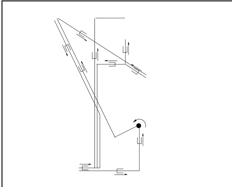
**Figure 4.11** Adding joints representing independent variations for the stacked blocks assembly.
