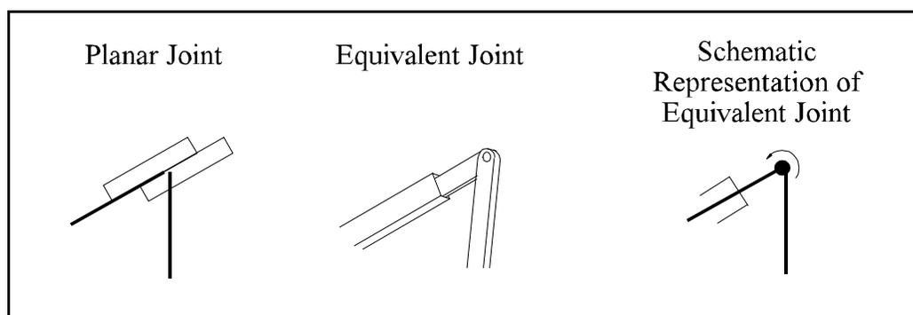
**Figure 4.12** The planar joint.
