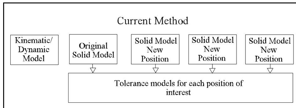
**Figure 1.1** Current techniques used for modeling tolerance and kinematic/dynamic properties of mechanisms.
