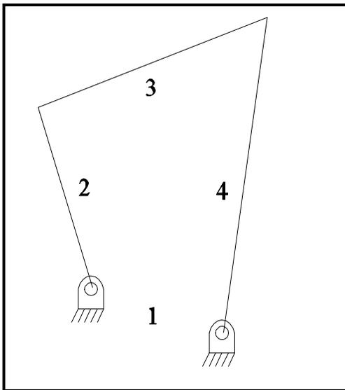
**Figure 2.1** A four bar mechanism.
