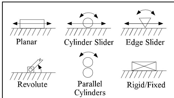
**Figure 4.5** Kinematic joints and their associated degrees of freedom.
