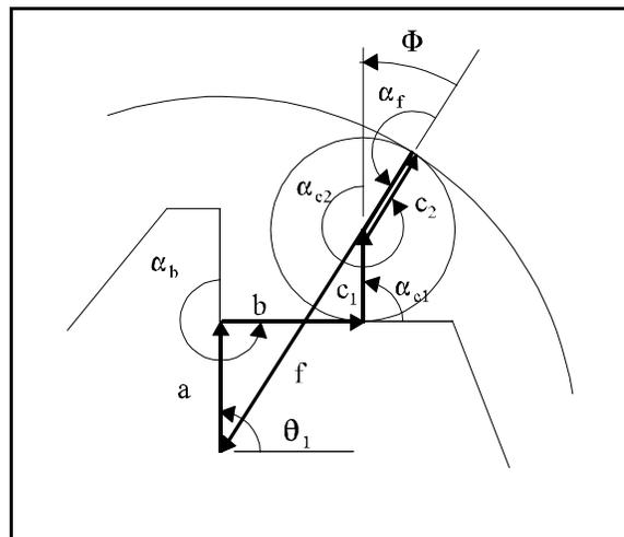
**Figure 3.3** The vector loop used to solve the clutch tolerance problem.
