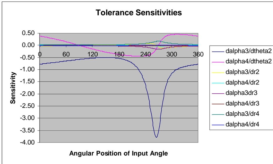
**Figure 5.16** Tolerance sensitivities for the full rotation of the four-bar mechanism.
