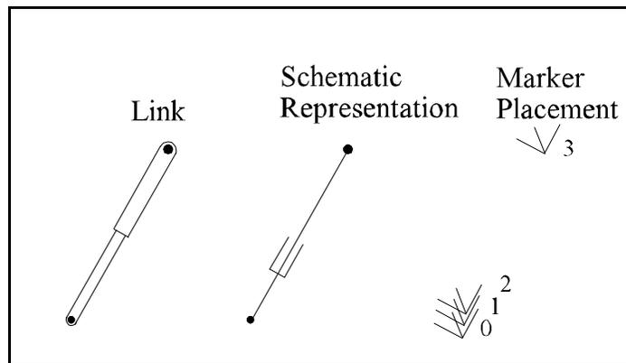
**Figure 5.8** Placement of marker on links with slider joints.
